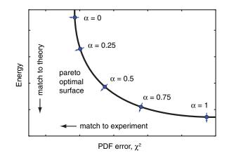
FIG. 2. Illustration of a combined optimization to match both theory (low energy) and experiment (small difference between the pair distribution functions). Optimization with different relative weights for these two objectives,  $\alpha$ , correspond to points on the pareto optimal surface.
