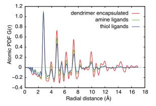
FIG. 1. Pair distribution function data of dry 1.7 nm Pt particles from total x-ray scattering. Dendrimer encapsulated particles have more order than particles capped with ligands, especially at lengths on the order of the diameter of the particle.
