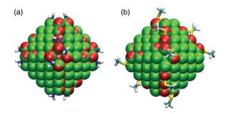
FIG. 7. Surface distortions in nanoparticle structure in ligand-bound nanoparticles (red) as compared to bare (green) particles: (a) 13 amine and (b) 12 thiol ligands.
