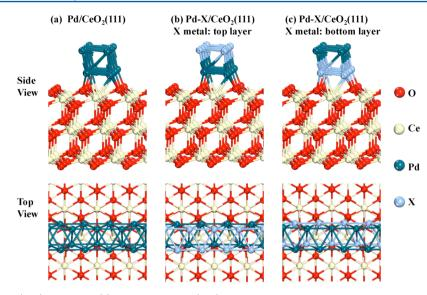
Figure 1. Structures of  $CeO_2(111)$ -supported (a) Pd nanorod and (b, c) bimetallic Pd–X nanorods where the X metal is in the top and bottom layers, respectively.
