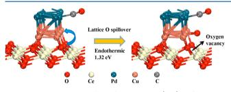
Figure 8. Lattice oxygen spillover from the  $CeO_2(111)$  surface to the Cu layer.
