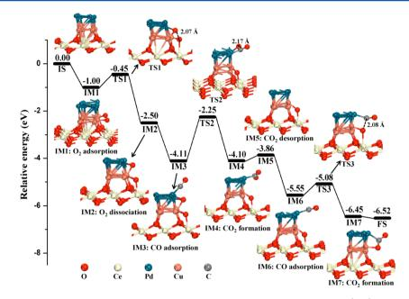
Figure 7. Calculated structures and energy profile in the direct O<sub>2</sub> dissociation pathway on Pd-Cu/CeO<sub>2</sub>(111).
