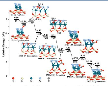
Figure 4. Calculated structures and energy profile in the direct O2 dissociation pathway on Pd-Ag/CeO2(111).
