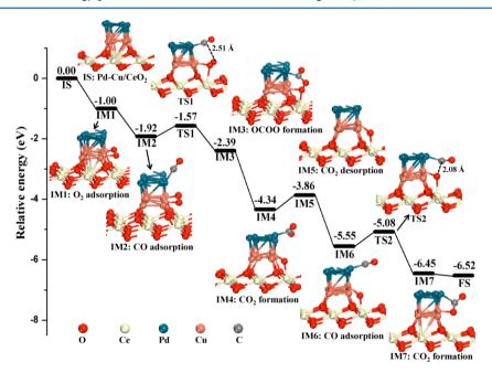
Figure 6. Calculated structures and energy profile in the CO-OO association pathway on Pd-Cu/CeO<sub>2</sub>(111).
