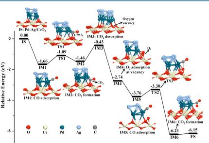
Figure 5. Calculated structures and energy profile in the M-vK mechanism on Pd-Ag/CeO<sub>2</sub>(111).
