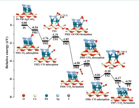
Figure 3. Calculated structures and energy profile in the CO-OO association pathway on Pd-Ag/CeO<sub>2</sub>(111).
