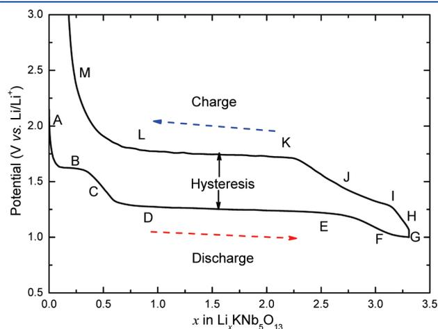
Figure 3. Behavior of lithiation and delithiation in  $\text{KNb}_5\text{O}_{13}$  at a current of 20 mA/g. Points A–M denote the  $\text{KNb}_5\text{O}_{13}$  state corresponding to the XRD and Raman testing.
